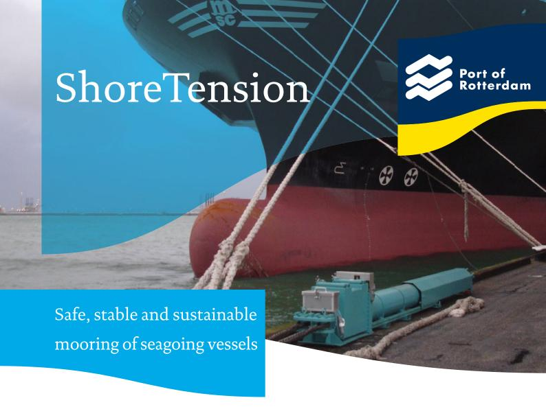
ShoreTension is a revolutionary system that prevents the breaking away of seagoing vessels from their moorings and ensures a more stable position in high winds and/or swell. Because ShoreTension is better able to hold ships in a stable position than their own mooring systems, it ensures higher productivity and less downtime of the terminal. Furthermore, important cargo handling equipment, such as (container) cranes, deep loaders and manifolds, is better protected.
